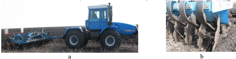
Fig. 6. General view (a) and working bodies of the experimental prototype (b) of the disc harrow DL-5 with the tractor XTZ-17022
