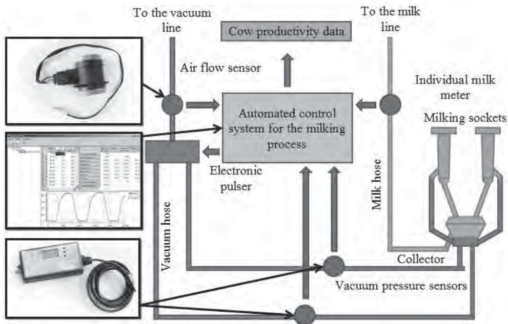
FIGURE 2. Automated control system for technical milking process
